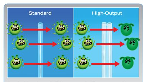
Standard Low-Output UVC lamps can only kill germs on surfaces inside your HVAC system, while High-Output UVC lamps can kill on these surfaces as well as sterilize airborne viruses, bacteria and germs as they pass by the lamp, rendering them harmless and incapable of reproducing.
