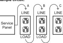
Placing the GFCI in the position A will also provide protection to the "load side" of receptacles B and C. On the other hand, placing the GFCI in the position C will not provide protection to receptacles A or B. Remember that receptacles A, B and C can be in different rooms.
