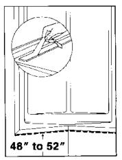
Remove backing from factory applied pressure sensitive tape.
