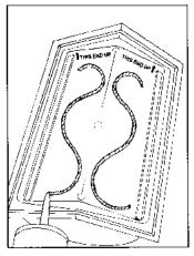
Apply a 1/8" bead of adhesive as illustrated. Keep adhesive at least 1" away from factory applied pressure sensitive tape.
