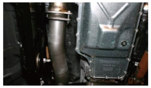
4. Next, install 61114NB pipe, placing hanger onto the OEM rubber mount and bolting the flanges together at the rear end.
