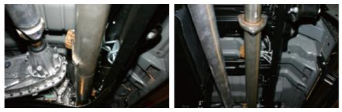
5. Next, install 61114NB pipe, placing hanger onto the OEM rubber mount and bolting the flanges together at the rear end.
