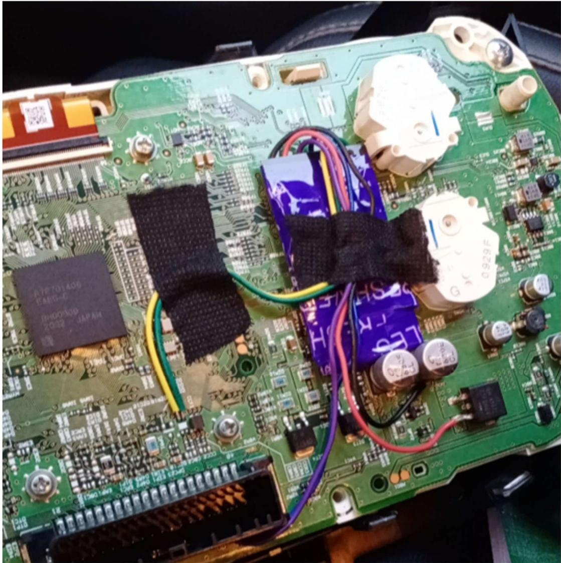
**4: Solder the filter according to the wiring diagram provided, Install dash on to car after soldering is completed.**
