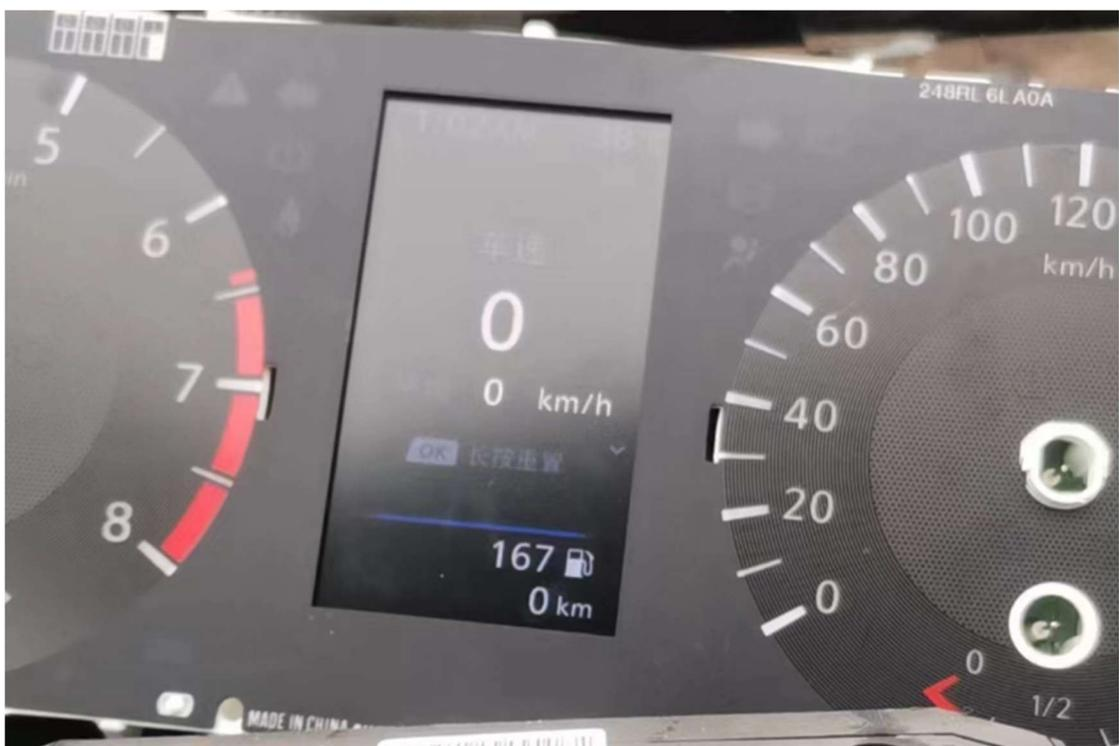
**5: When the dashboard is installed on the car, the dashboard shows 0KM, and after driving 1KM on the road, it will be the mileage you want.**
