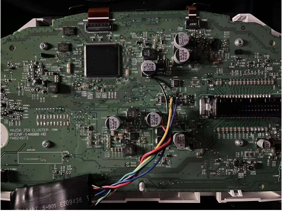
4: Solder the filter on dashboar according to the wiring diagram provided, Install dash on to car.
