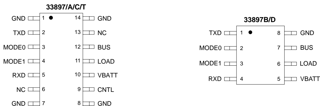
Figure 4. 33897/A/B/C/D/T Pin Connections
