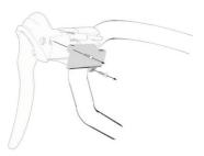
**2E.** Insert the Archer DBR remote in the shallow recess on the inside of the brake lever. Use the two Torx T6 screws that held in the hydraulic cap to affix the DBR into place. Tighten to 2Nm.
