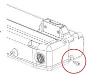
Close the battery door and tighten the screw.
