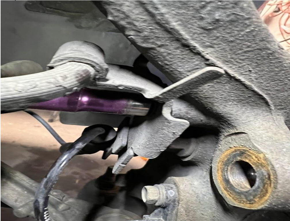
Step 4: Disconnect brake hose from knuckle & chassis
