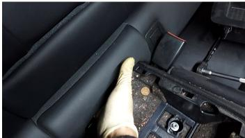
10. Now with both versions of the rear console cover removed you will have access to the factory plug that powers the 12v lighter plug. This is the plug you will use to connect our wiring harness to.
