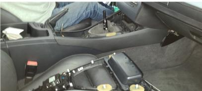
4. With the console trim upside down locate the 4 t10 torx screws and remove with included tool. (Only applicable for cars with smokers package ashtray / induktiv unit with tray
