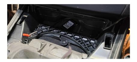
Plug the converter and charger into each other. Finally reinstall console trim, shifter surround and shifter / shift knob.
