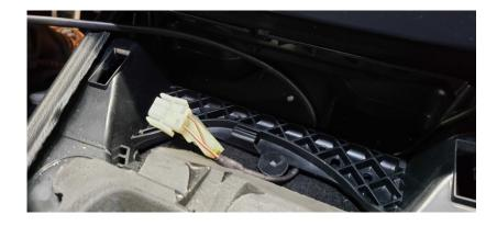
6. Continue routing the harness toward the ebrake area tucking it next to the shifter as shown.
