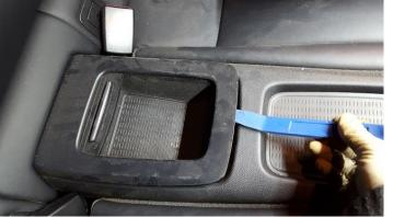
Once removed locate and remove the 2 10mm nuts. Now grab the seat panel and remove also.
