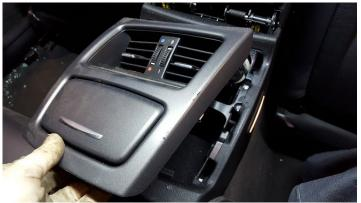
Once removed locate and remove 2 T20 screws. Now you will move onto the rear tray / pad. Remove the same way as the vent piece by prying up.
