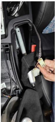
8. Now route the cable down the inside of the console towards the floor of the vehicle and out the bottom of the center console.
