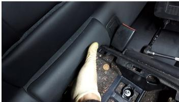
10. Now with both versions of the rear console cover removed you will have access to the factory plug that powers the 12v lighter plug. This is the plug you will use to connect out wiring harness to.
