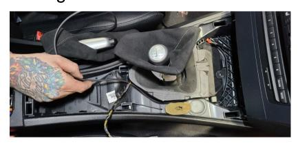
7. Pull up on the front edge of the ebrake boot to lift up. This will help in routing the wiring harness towards the rear of the center console.
