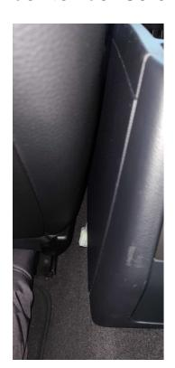
9a. E90 / E91 cars the rear of the console has a cover that unclips and pulls off. Move to step 10.
