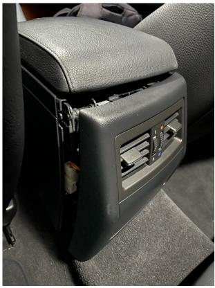
9b. E92 / E93 cars the rear console is extended to the rear seats. First remove the panel with the vent by prying up from the bottom.
