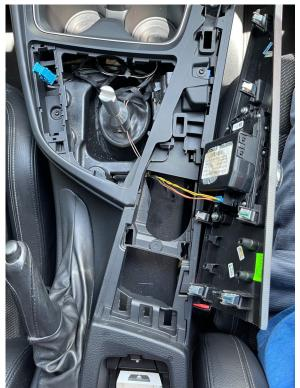
5. Now take the Included T20 Allen tool and remove the x2 t20 Allen screws shown below.
