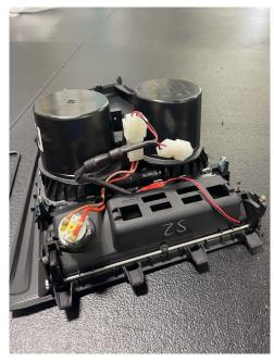
11. Make sure the lid works properly by lifting up and checking to see if it holds itself open. If everything works as it should you can now re install the console back in the vehicle doing steps 6-1 in reverse order.
