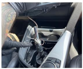
2. Now that the shift knob and boot is removed next you will lift up the traction control button by reaching to the front with your middle or ring ringer and pushing the clip all the way at the front towards the rear of the car and up and it will release upwards. Remove plug and place to the side.
