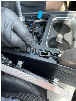
6. After the x2 T20 screws are removed, you will now start lifting the console to get it ready for removal. Once you have it lifted you will remove the small black and the white colored lighter connector shown below. Once done remove console.
