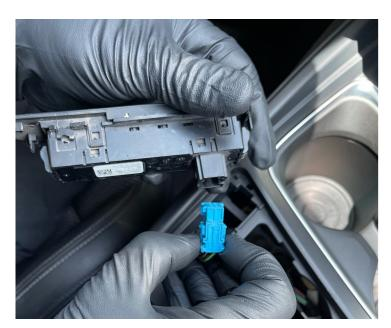
4. Next you will need to remove the trim on the side with the idrive controller. First lift the armrest, next you will need to use a pry tool or your fingers to grab an edge and lift the trim up. Once lifted you will flip over and leave to the side.
