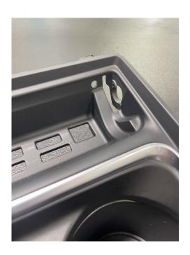
10. Now with the hole drilled run the red connector through the hole. Once ran you will install the new Induktiv charging lid using the same 2 springs, black clips and metal bar.
