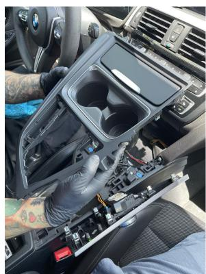
7. With the console removed we can move onto installing the wireless charging unit. 1st we will remove the 2 springs on each side. Followed by the 2 plastic clips using a small screwdriver or pick. Finally you will need to remove the long metal bar. (We will use in next step)
