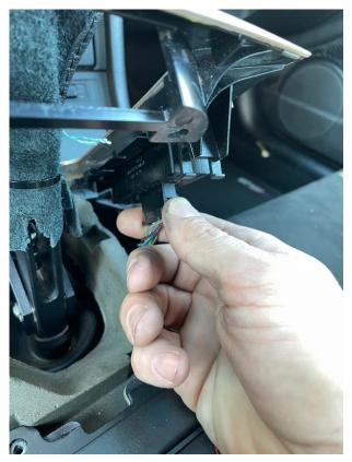
4. With the console trim unplugged and removed you now will access and remove 4 Phillips head screws to allow access to the 12v lighter plug and harness which we will use to power the charger. Open the lid to the storage tray and pull straight out. If you have heater controls you will need something to pry.
