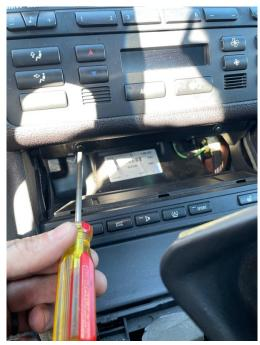
8. Next you will lift up the trim piece to access the bottom of the 12v lighter and un plug the 2 factory plugs shown below. You will then plug our harness into the lighter plug and finally plug the other ends of our harness into the factory plugs
