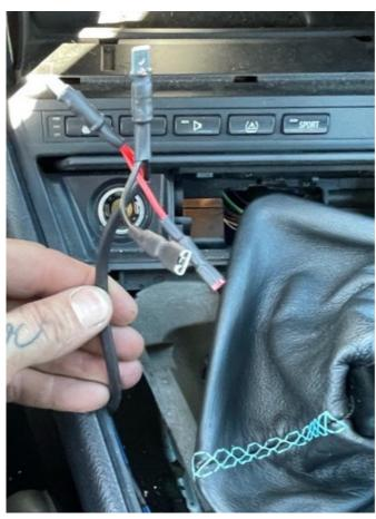
7. With the harness run, you will now loosen the 4 Phillips screws we mentioned in step 4. Location shown below
