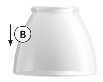
A. Pull the cover down on to the frame. Adjust it so that the silicone lip covers the bottom of the frame evenly around.
