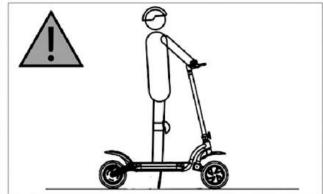
DO NOT stand on the footboard after the scooter is powered off and stops.
