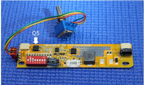
Note: When using an external brightness control, no connection on pin 4 (ADJ)
