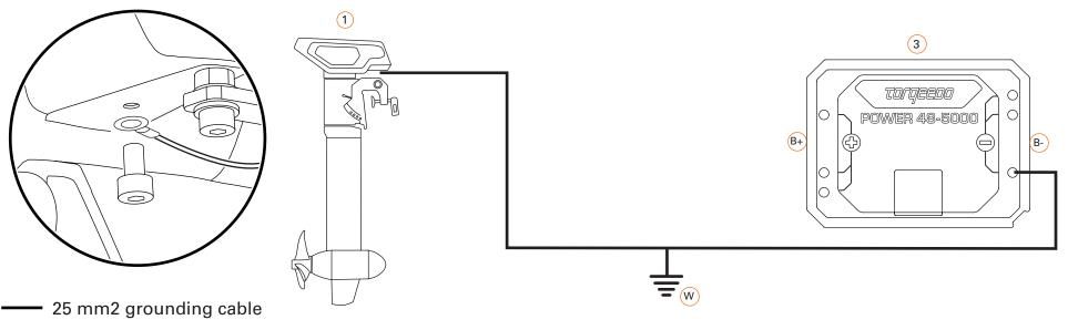
Installation Drawing: I13 Version 1.1 System ground connection
