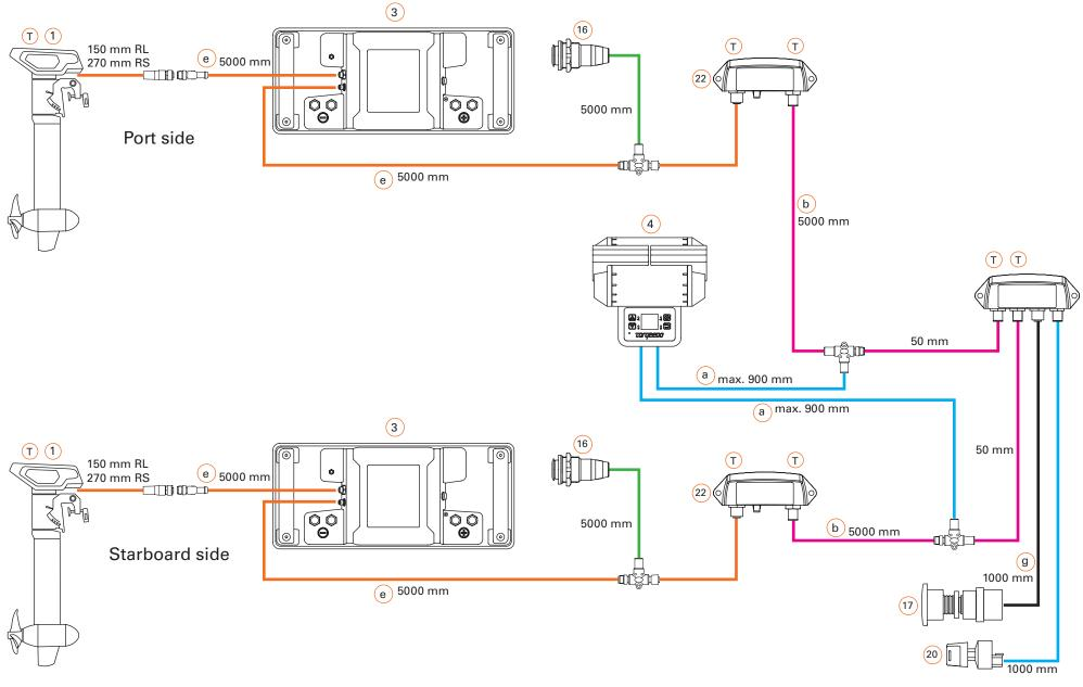
Backbone TorqLink, 8 pin data cable
