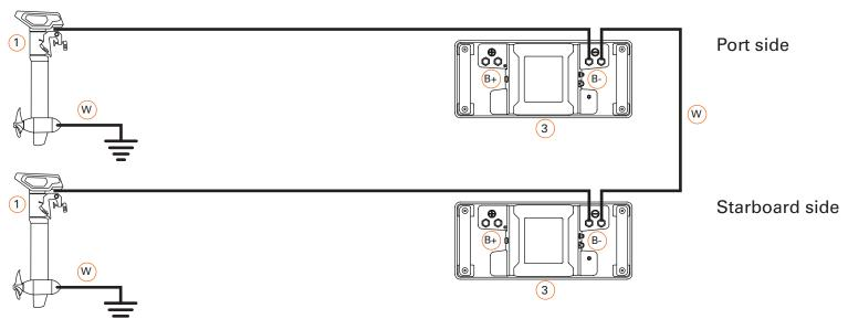
In this configuration the motor fullfills the function of the grounding point
