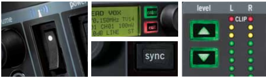
Left: RF Mute Switch prevents RF transmission during setup Top middle: Easily navigable grouped LCD menu Bottom middle: Scan & Sync vastly improves setup efficiencies Right: Input level adjustment and LED meter
