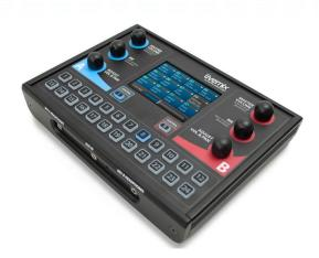
MirrorMix<sup>™</sup> function allows you to use your own personal mixer to listen to and adjust the mix of any other personal mixer in the system. Even though it is designed to be simple to operate, we did not skimp on the features, like built-in ambient mics, effects on every channel and even a metronome.
