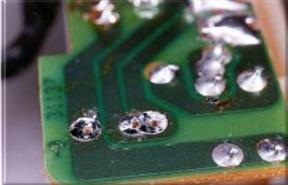
**(Left)** The faulty electrolytic capacitor dropped out of the board after desoldering. Sometimes, it may need persuading with pliers.... but don't overdo this or you risk damaging the copper tracks on the p.c.b.
