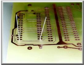
(**Left**) A useful product is Multicore's Tip Tinner Cleaner (TTC) - a 15 gramme tin of special paste which cleans and "tins" the soldering iron iron, in one go. New tips must be tinned **immediately** when used for the first time. (**Right**) Insert components and splay the leads so that the part is held in place.
