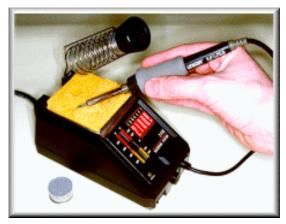
(**Left**) Printed circuit board copper tracks must be clean to begin with, especially if they're not previously "tinned" with solder. Clean any raw p.c.b. copper tracks gently with e.g. an abrasive rubber block available from electronics suppliers. (**Right**) Clean the iron "bit" (soldering iron tip) using a damp sponge. The soldering iron featured is an Ungar Concept 2100 Soldering Station. Other popular brands of soldering equipment include Weller and Antex.
