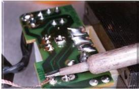
**(Left)** Select a suitable width of desoldering braid, and **press it down** onto the **COLD** joint using the hot tip of the iron. A flat soldering iron bit is preferable.
