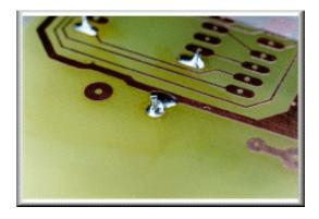
An example of a "dry" or "gray" soller joint - the solder failed to flow, and instead beaded to form globules around the wire.
