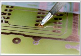
(**Left**) It's usually best to snip the electronic component wires to length prior to soldering. This helps prevent transmitting mechanical shocks to the copper foil.(**Right**) Apply a clean soldering iron tip to the copper solder pad and the component lead, in order to heat *both* items at the same time.
