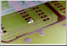
(**Left**) Continue heating and apply a few millimetres of solder. Remove the iron and allow the solder joint to cool naturally. (**Right**) It only takes a second or two, to make the perfect joint, which should be nice and shiny. Check the Guide for troubleshooting help.
