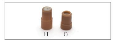
**Changeable Caps:** Change the polar pattern from hypercardioid to cardioid by swapping the plastic protective cap. Use hypercardioid for maximal isolation, and cardioid for a wider front-lobe (more flexibility in mic placement).
