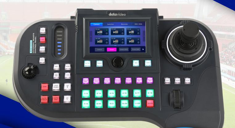
RMC-300A is a multi-functional multi-camera controller. It is able to control up to 12 PTZ and block cameras by Ethernet and up to 8 cameras by serial port RS-422 transmission. The RMC-300A versatility allows you to control Datavideo PTZ cameras, robotic PTZ heads and switchers up to 12 channels via serial RS-422 or IP control. A user friendly GUI combined with a 5" touch panel control and tactile control buttons enable users to manage multiple cameras for larger productions.
