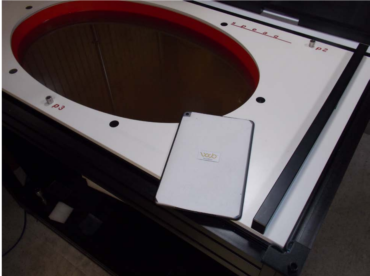
iPad with WaveBlock on Test System
