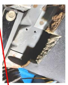
For reference, the original dimmer knob was located here: —— Wanting to make the installation as "invisible" as possible, I painted the surface of the bracket that faces the driver position black then mounted it using the two screws that formerly held the factory rheostat!
