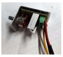
Next, came the "how to install" thoughts. Holding the bracket and module assembly up to the area near the factory rheostat location revealed some of the dashboard material would have to be removed to allow mounting the assembly by way of two screws; the added holes can be seen in the third image:
