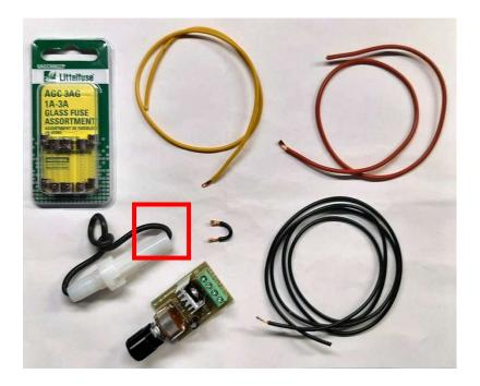
The "U" shaped wire section in the red box above is a "jumper" that goes between the two negative connections on the module. This was a result of confirming with the vendor that the "chassis" ground was an acceptable connection for the output side of the module thereby being compatible with the single wire dash light configuration. Here the module with the jumper and ground wire attached:
