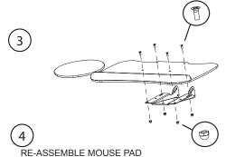
RE-ASSEMBLE MOUSE PAD AND APPROPRIATE MOUSE FENCE
