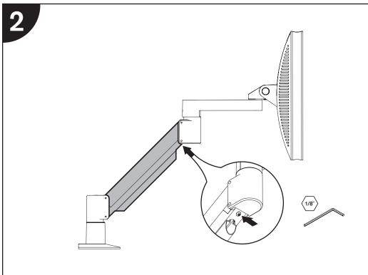
In some instances, an additional counterbalance adjustment may be needed to allow the arm's instant height adjustment function to work properly.
