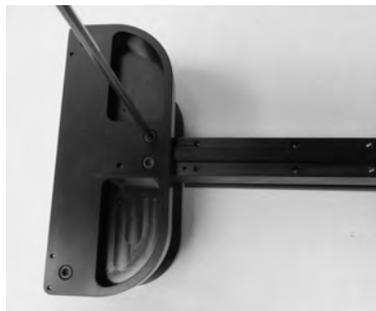
D. Install the Trigger Catch on the end of the Operation Rod where it engages the original AR15 Trigger. It requires a 5/32" Allen Wrench for the 8-32-½" screw. Do not tighten until the Trigger Catch is adjusted. [See Photo on Following Page.]
