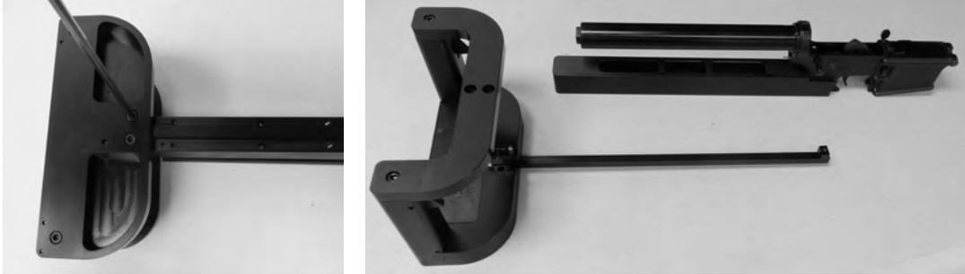
I. Unscrew the  $\frac{1}{4}$ -28-1" Grip Screw from the Lower Receiver Extension and AR15 Receiver.
