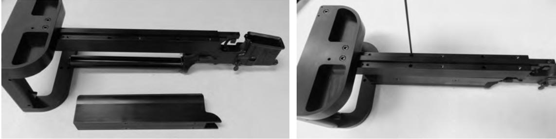
**F. Hold the Clam Shells in position while screwing the Lower Receiver Extension to the Clam Shells. Install four 6-32-1" screws with the 7/64" Allen Wrench.**
