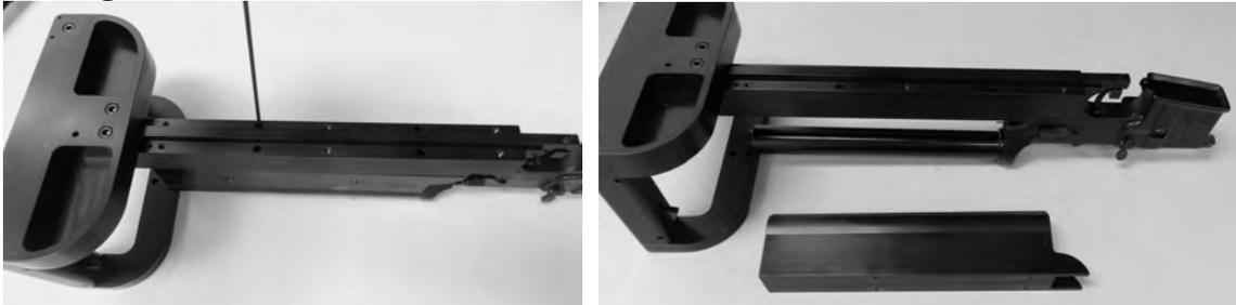
H. Unscrew the two  $\frac{1}{4}$ -20-1" screws holding the Bottom Plate of the Spade Grip Assembly to the Lower Receiver Extension with a  $\frac{3}{16}$ " Allen Wrench.
