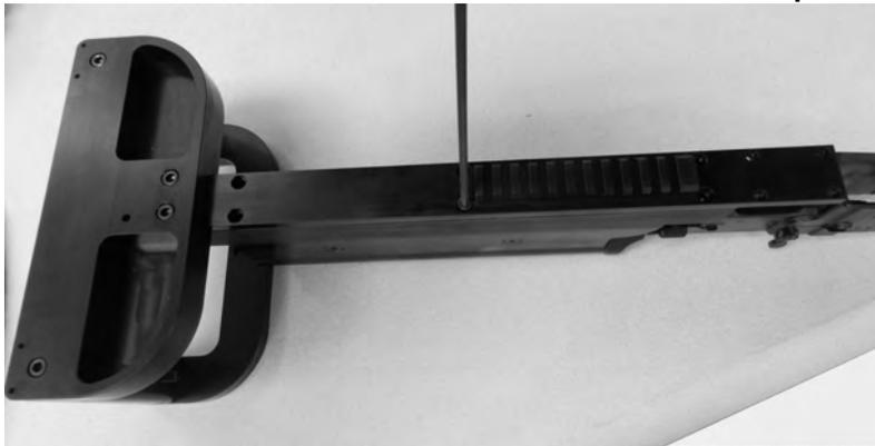
**C. Loosely screw in the six 10-32-1/2" screws that hold the Base Plate to the Lower Receiver Extension.**
