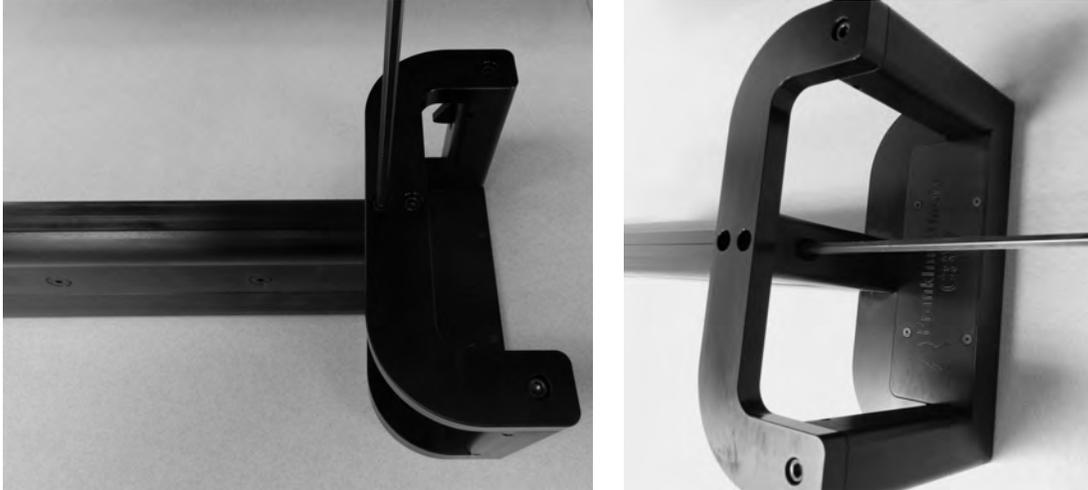
B. If your CSW™ is attached to a firearm, unscrew the singular  $\frac{1}{4}$ -28-1" screw that attaches the Column Block to the Receiver Extension with a  $\frac{3}{16}$ " Allen Wrench.
