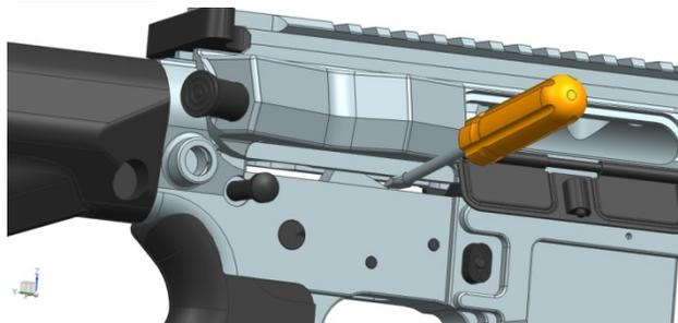
Be careful to not pull the Upper and Lower apart so tightly that it binds the Carrier in between the two as this may prevent the Carrier from moving forward even if the Hammer is appropriately clear of the Carrier. In addition, be careful not to mar the finish of the Upper or Lower Receiver.
