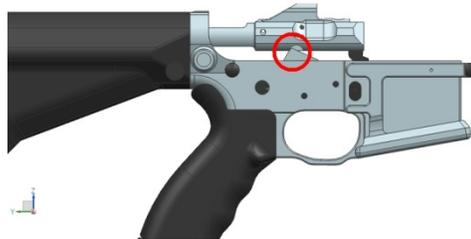
**Warning:** Do not attempt to cycle the action of the F17-VS4™ if your Buffer is seated *deeper* than  $2-37/64''$  (or 2.578'') The Carrier may cycle far enough rearward that it will get caught on the Hammer, preventing it from traveling forward. **See Figure D.**
