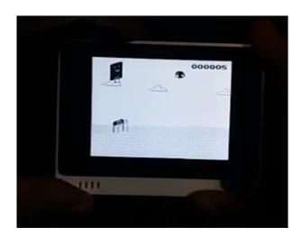
**Step 2**. To install the P25RX display firmware, the WioTerminal must be in "bootloader" mode. Quickly slide the power switch down twice (like double clicking a mouse). The screen will be blank and the blue LED near the USB port should be "pulsing" when in bootloader mode. It may take a you few trys to get the power switch slide timing correct.
