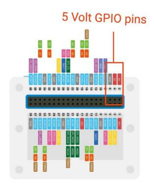
Q: Why do I need to power the Wio Terminal through the back GPIO pins?
