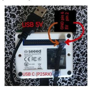
Here is an example from the internet using power pins to a screw terminal block jack.
