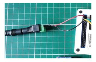
Like above, this is a USB screw terminal cable solution example.
