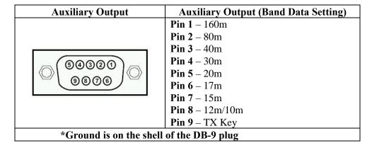
When the transceiver or antenna is selected for a particular band. The pin on the Auxiliary Output jack will corresponding to the band will be 5V. When using UHF/VHF the output from the Auxiliary Output port will be as follows:
