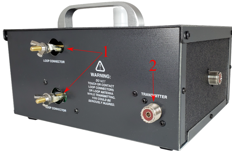
Figure 5: Rear-panel Connections: 1.) Wire loop connectors, 2.) Coax input
