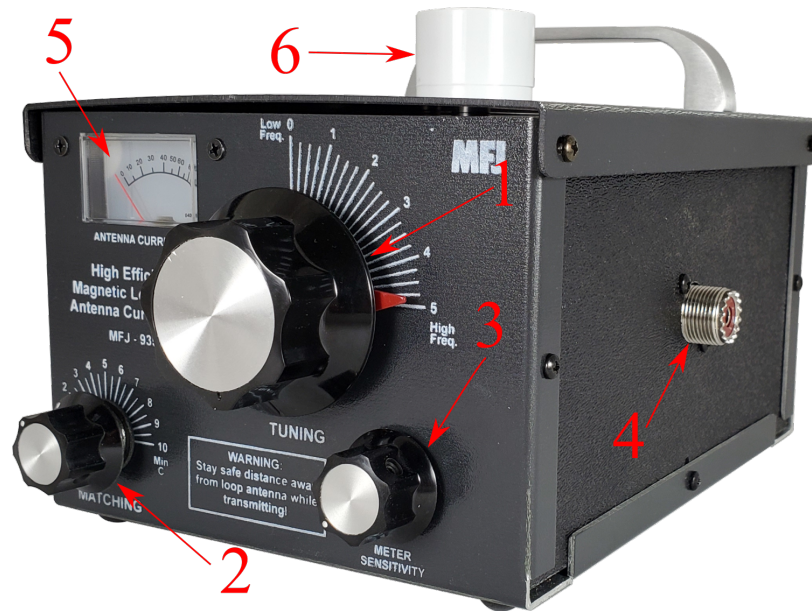
Figure 4: Front-panel Controls: 1.) Tuning Control, 2.) Matching Control, 3.) Meter Sensitivity, 4.) Coax Output, 5.) Antenna Current Meter, 6.) PVC Mount
