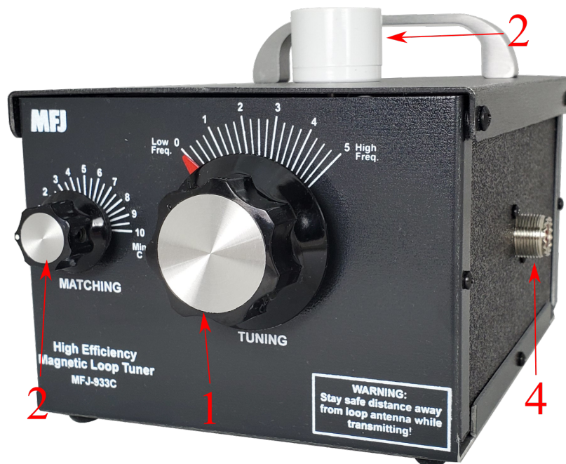
Figure 4: Front-panel Controls: 1.) Tuning Control, 2.) Matching Control, 3.) PVC Mount, 4.) Coax Output
