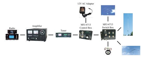
Figure 4: MFJ-4713 Station Setup
