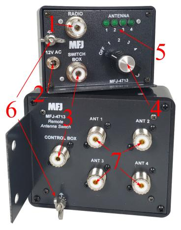
Figure 3: MFJ-4713 Controls: 1.) To Radio, 2.) 12V AC input, 3.)Box Link, 4.) Antenna Selector, 5.) Antenna Indicators, 6.) Safety Ground, 7.) Antenna Ports.
