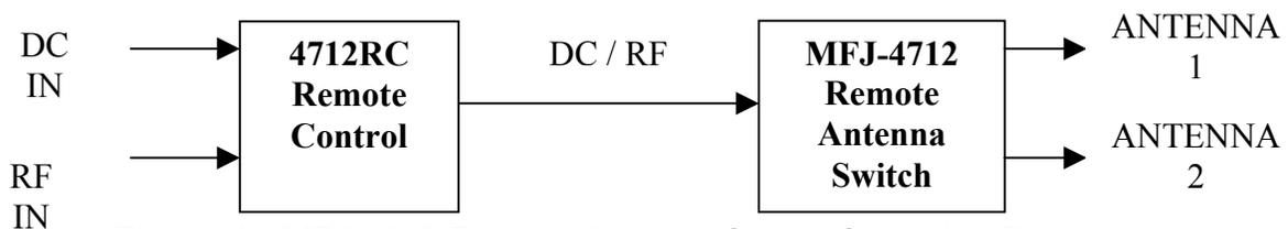
**Figure 1:** MFJ-4712 Remote Antenna Switch Operation Diagram
