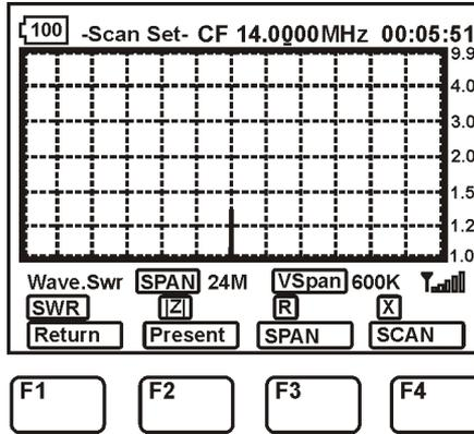
In *Scan-Set* mode, the four function keys are assigned the following functions:
