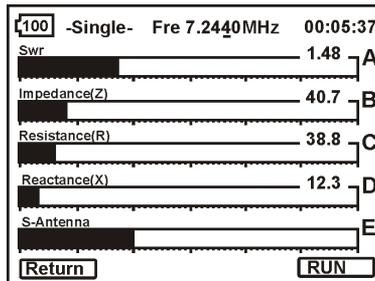
With the generator running, you may change frequency on the fly using the *Encoder* while watching the display for key points of interest such as resonance ( $X = 0$ ), minimum *SWR*, and the antenna's 2:1 bandwidth limits. You may also use the analog bars to provide continuous feedback when adjusting tunable circuits or matching networks. Pressing Run/Stop again toggles the generator off.
