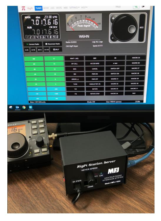
RigPi Station Server (RSS) is a computer system designed to control your station and facilitate on-the-air activities. RSS introduces a radically new way of station control by using a server model for allowing multiple users and radios to be accommodated simultaneously through standard Internet browsers.
