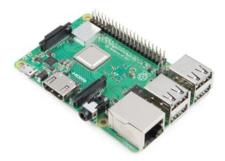
RSS is based on a Raspberry Pi computer running Linux plus RigPi Keyer and RigPi Audio boards. RigPi Keyer uses the popular K1EL WinKeyer chip for keyboard or paddle input. RigPi Audio is used for Voice-Over IP (VoIP) and remote operations, or for digital modes and I/Q spectral display (panadapter).
