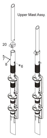
Slip the upper mast assembly and the 1.25" hose clamp (20) into the loading coil assembly and align the holes then slide the 6-32x1.5 SS screw (7) and #6 lockwasher (8) through the holes and the solder lug. Attach the 6-34 KEP nut (6) to the screw and tighten down. Tighten the hose clamp.
