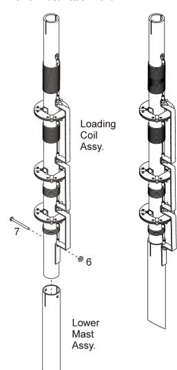
Attach the lower mast assembly to the loading coil assembly using 6-32x1.5 SS screw (7) and 6-32 KEP nut (6). Slide the mast assembly over the fiberglass tube and align the hole in the aluminum tube with the fiberglass tube. Slide the screw through the holes and attach the nut. The solder lug will be between the aluminum tube and the jumper bracket. Tighten the nut and screw.
