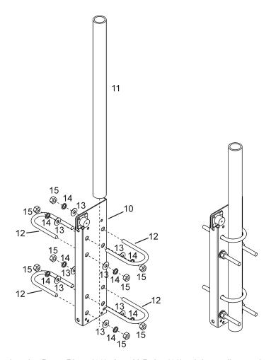
Assemble the base using the Base Plate (10), four U-Bolts (12), eight  $\frac{1}{4}$ " flat washers (13), eight  $\frac{1}{4}$ " lock washers (14), and eight  $\frac{1}{4}$ -20 nuts. Loosely attach the U-Bolts then slide the fiberglass base insulator (11) into the U-Bolts as shown in the picture and tighten up the U-Bolts holding the fiberglass base insulator.
