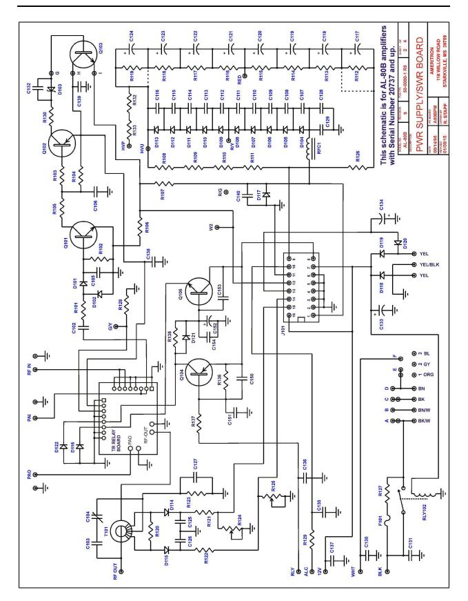
Figure 6 Power Supply / SWR Board
