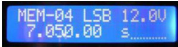
Click this button will be Alternating between Memory mode(MEM)and VFO mode, the LCD screen will show the MEM-\*\* or VFO-\*\*(The figures for 01-30).In Memory Mode the Tuning knob is used to change memory locations. In VFO Mode the Tuning knob is used to change the frequency.
