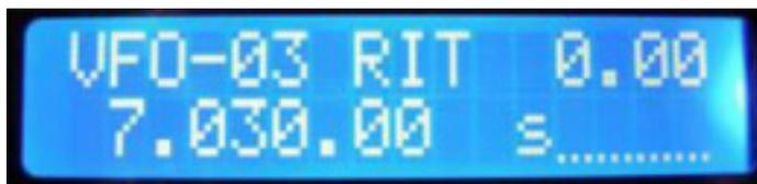
Click this button to enter or exit RIT function. RIT 0.00 showing, the step is 10Hz in adjustment mode
