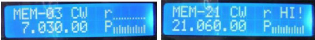
You can transmit in 5 mentioned band. The screen display “TX” when transmitting. S meter indicate the power output, screen showing forward power output and R for resistant power, you want to see less R as possible. Showing HI! Means your SWR is too high to operate. The indicator closed to antenna showing light up means in transmitting. The screen display “TX ERRER” when you try to transmit outside 5 Ham band.
