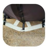
Locate the buckles under your hull, unclp the buckles, wrap the webbing around your bunk bar, re-clip the buckles and adjust the straps to be snug.
