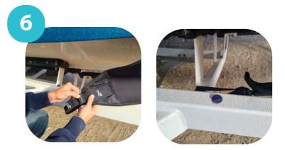
Take your side trailer support straps, un-clip the buckle and wrap the webbing around your trailer bunk bar, re-clip the buckle and adjust the straps to be just snug.
