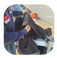
Take both sides of the end of the zipper (where the winch post hole is) and wrap it around your winch post.
