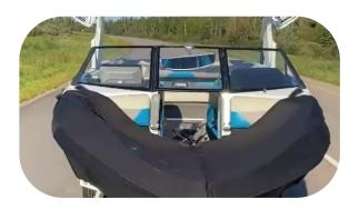
**IMPORTANT** You want the center of the bow panels to come down and the neoprene to wrap down the inside of the side of the bow so air does not get under the cover. You want the cover to be tight and not loose. If you notice significant flapping, stop immediately and adjust the bow strap so there is not too much air force on the shield.
