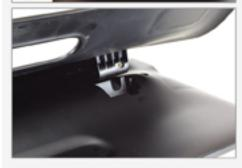
(c). Push the latches toward one another and pull the stand away from the back of the tablet.
