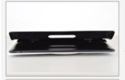
(a). Lay the tablet face down and locate the two spring-lock mechanisms where the stand attaches to the tablet.
