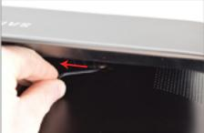
(b). With the included allen key, insert the tool in to the holes on the latch.
