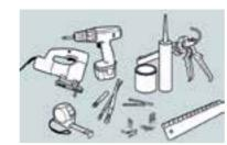
Screwdriver with different tips for screws Electric saw with wood cutting blade (a radial arm saw is recommended for professionals) Cartridge Gun, Tape measure, Ruler, Paintbrush, brush for putty texturing, 3mm and 8 mm bits, Wall plugs & screws, Electric nail gun, Filler Putty one square meter. (indoor), Exposy putty (outdoor installation), Paint & aged spray
