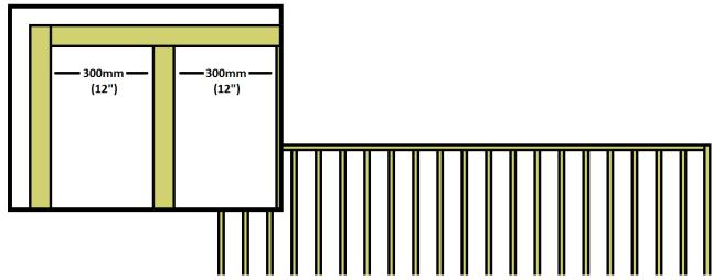
When building your timber sub-frame, we reccomend using nothing less than 4"x 2" (100mm x 50mm) timbers. This gives a good sturdy frame for your decking to fix to and is adequate for a deck either on the floor or upto a 2ft high elavated deck. If your deck is higher than 2ft from the floor then we recommend you upgrade your frame timbers to 6"x 2" (150mm x 50mm) as this will create a much sturdier base.
