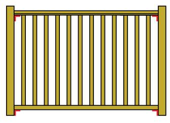
Spindles: When working out the quantity of spindles required, remember to include the size of the spindle. We generally recommend a 100mm gap between the spindles so by using the combined measurement of both the spindle and the gap,
