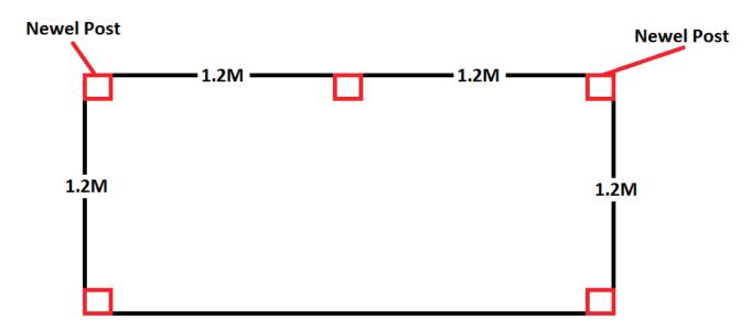
Always remember to include the width of the newel posts and spindles when calculating for the materials, this keeps cuts down to a minimum
