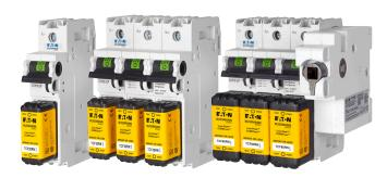
The DIN-Rail mounted 1-, 2- and 3-pole Compact Circuit Protector (CCP2\_CF) is a UL 98 horsepower rated disconnect available in 30, 60 and 100 A ratings. Each CCP will accept a fuse amp rating equal to or less than its rating. These switches are also available in rotary versions for through-the-door or through-the-side operation. Accessories include multi-wire lug kits with terminal shrouds, auxiliary contacts and PLC fuse monitor (see data sheet no. 1157).
