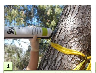
Beginning on the north side of tree, place the tip of the caulking gun squarely against the bark of tree at a height of six feet. Dispense a disc-shaped point source of approximately 2½ inches in diameter and ¼ inch thick.
