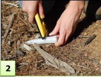
Cut applicator tip 1½ inches from base (at the point where the ridges end).
