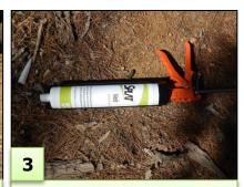
Screw the applicator tip onto the SPLAT Verb tube and place tube into a large caulking gun (contractor size).
