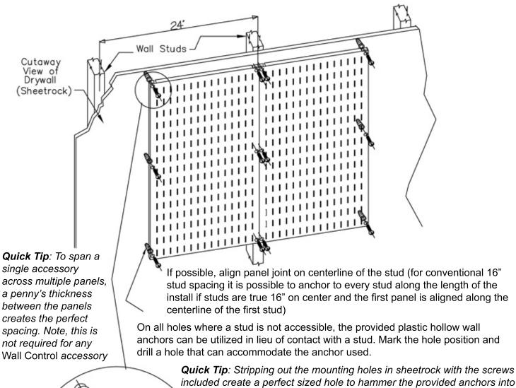
included create a perfect sized hole to hammer the provided anchors into
