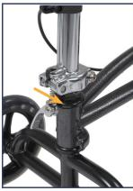
3. Slide locking mechanism into groove on tiller, press locking handle to secure tiller lock in place.
