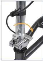
Insert pad post into receptacle on frame. Secure
