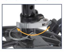
Attach basket by sliding basket receptacles down over hooks on the front of the tiller.
